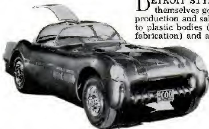
PACKARD displays its Panther, one of few plastic bodies built on a full-size chassis. It has a 275-hp. engine
